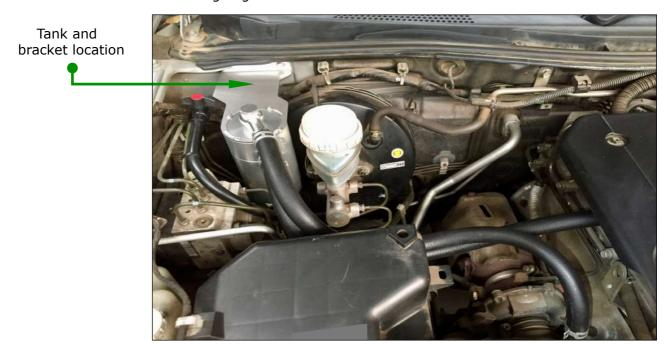
**NOTE:** SAAS recommends checking your catch tank after traveling 1000km to see how much oil has accumulated in the tank. It is important that the build-up of oil does not rise above the internal baffle through to the bronze filter.
