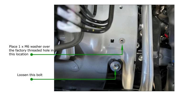
**Step 4:** Slide tank and bracket under the air box bolt. Fit  $1 \times M6$  bolt and washer (shown below) and tighten all bolts. If you wish to use the supplied drain valve, attach the drain valve to the tank before mounting to vehicle.
