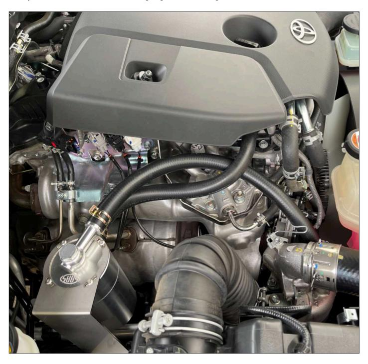
**NOTE:** SAAS recommends checking your catch tank after travelling 1000km to see how much oil has accumulated in the tank. It is important that the build-up of oil does not rise above the internal baffle through to the bronze filter.
