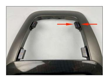
**- 4** Fit the dash bracket to the dash surround as show below using 2 of the factory screws.
