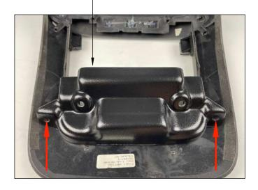
**- 5** Fit the dash surround to the vehicle using 2 of the factory screws to hold the top of the dash surround in position as shown below.
